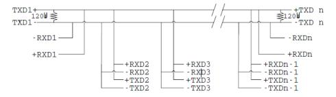
**Note:** BOTH ends of MAIN line terminated in characteristic impedance, stubs off main line not impedance, since both ends receive. The twisted pair ends are wired to both RXD+ & TXD+ and RXD- & TXD- at each RS-485 device!
