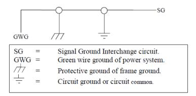
**Configuration A)** The circuit common of the equipment is connected to protective ground, at one point only by a 100  $\Omega$ ,  $\pm 20\%$  resistor with a power dissipation rating of 1/2W. An additional provision may be made for the resistor to be bypassed with a strap to connect signal common and protective ground directly together when specific installation conditions necessitate.
