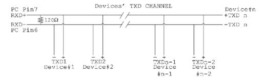
**Note:** The receiver end of MAIN line terminated in characteristic impedance, stubs off the main not terminated.
